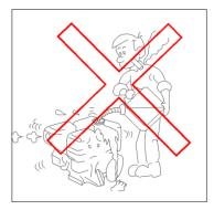
and do not use leaded gasoline, fake gasoline, or denatured gasoline. It adversely affects each part of the engine and leads to engine trouble or breakdown.
