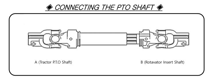
1. Ensure that the universal joints at each end of the PTO shaft are in alignment as shown in the drawing.
