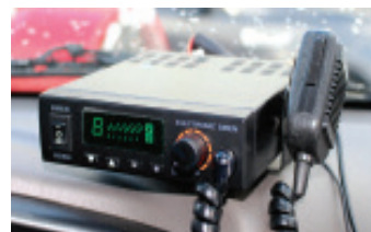
Amp and warning light control box
