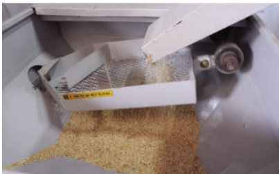
Built - in screening and foreign substances screening network
