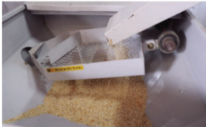
Built - in screening and foreign substances screening network
