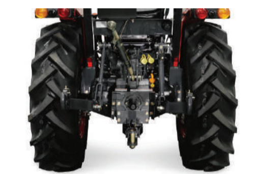
The Category I hitch has a lift capacity of 1,500kg at the ball end and 1,100kg measured 610mm behind the ball.
