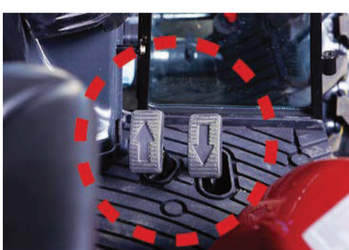
Hydrostatic control pedals for smooth hands free forward reverse motion HST models
