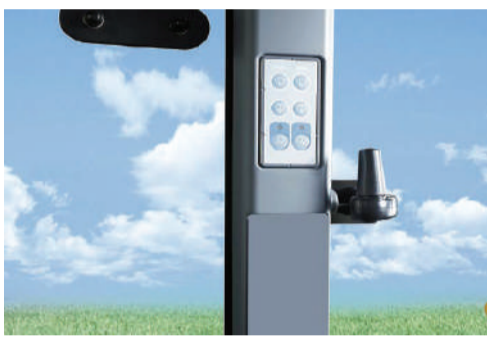
Easy access to the button type light controller located on the inner pillar of cab.
