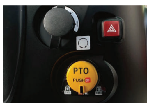
PTO operation : Electric Hydraulic Independent or Clutch linked
