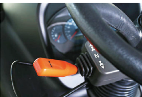
Power shuttle lever enables easy shifting between forward and reverse.
