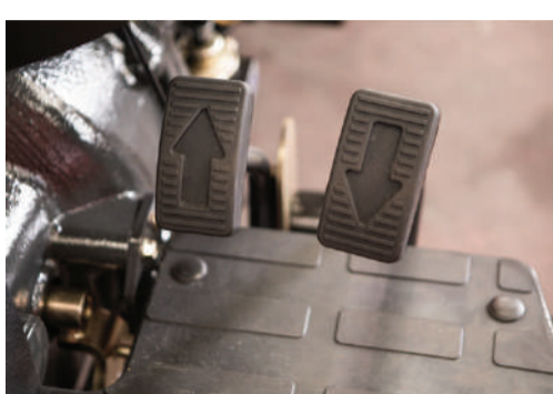
Dual hydrostatic control pedals for smooth Forward / Reverse (only for HST model)
