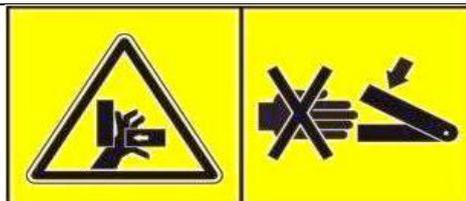
Be extremely careful handling various parts of the machine. They are heavy and hands, fingers could be crushed or pinched between tractor and implement
