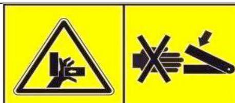
Be extremely careful handling various parts of the machine. They are heavy and hands, fingers could be crushed or pinched between tractor and implement
