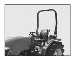
The safety frame is intended to reduce damage of an accident in case of a rollover, so it cannot prevent an accident
